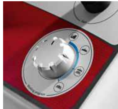
User friendly control panel with working program selector, forward / backward gear selector and emergency button
