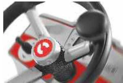
User friendly control panel with working program selector, forward / backward gear selector and emergency button
