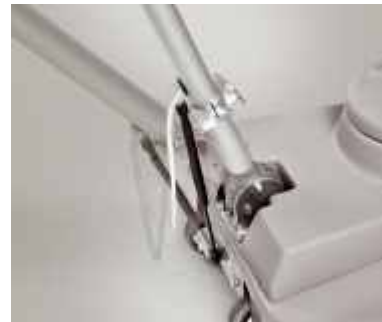
Gas spring assisted system which ensures disc pressure on the floor is kept constant regardless of the drive handle position. In this way the surface does not get burned or damaged
